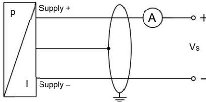
**NOTE** - Use a shielded and twisted multicore cable for the
