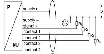
**NOTE** - For the electrical connection, a shielded and twisted multicore cable is recommended
