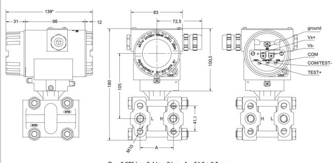
$\begin{array}{l} P_{N} = 0.075 \; bar, \; 0.4 \; bar, \; 2 \; bar \; : \; A = 54.5 \pm 0.5 \; mm \\ P_{N} = 7 \; bar & : \; A = 56.0 \pm 0.5 \; mm \\ P_{N} = 20 \; bar & : \; A = 56.5 \pm 0.5 \; mm \end{array}$
