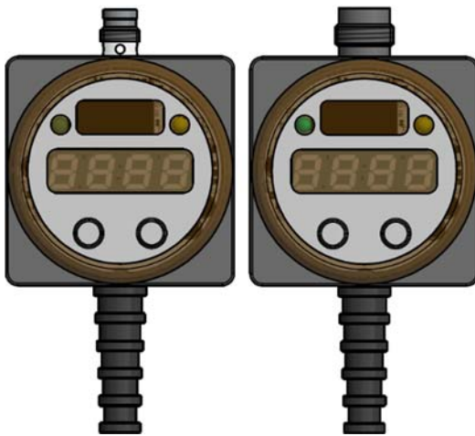
M8x1 and M12x1 (4-pin) male connector
