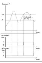
Fig. 4 Switching and resetting behavior for hysteresis function in pressure-time graph
