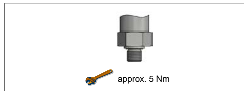
Fig. 2 connection G1/4" according to DIN 3852
