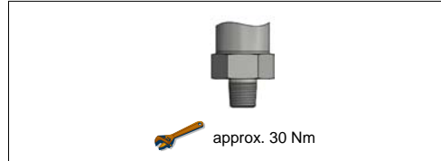
Fig. 3 connection 1/4" NPT
