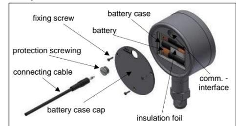
Fig. 3 Battery case and communication interface
