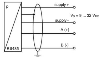
RS 485 / Modbus RTU with reset function for DCT 531, DCT 531i, DCT 531P, DCT 561 und DCT 571
