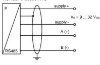
RS 485 / Modbus RTU with reset function for DCT 531, DCT 531i, DCT 531P, DCT 561 und DCT 571
