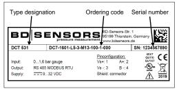
Fig. 1: Example of manufacturing label
