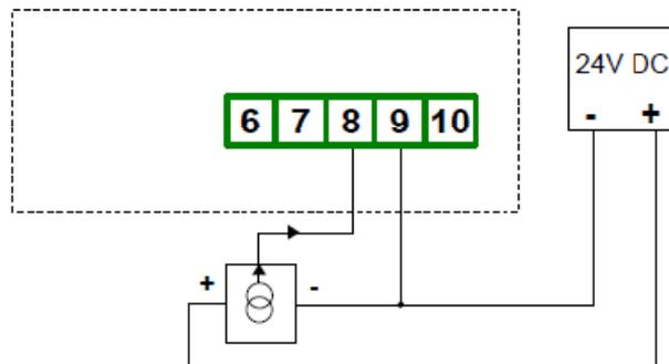
Fig. 4.8. connection of 3-wire current converters
