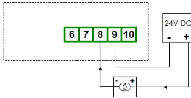
Fig. 4.7. connection of 2-wire current converters
