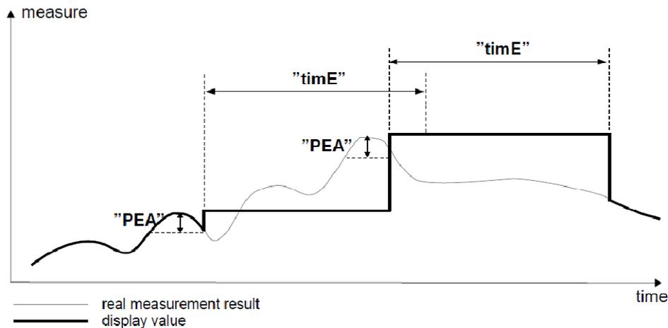
Fig. 6.3. process of peaks detection
