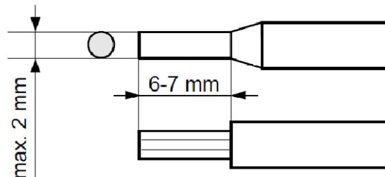
Fig. 4.4. method of cable insulation replacing and cable terminals
