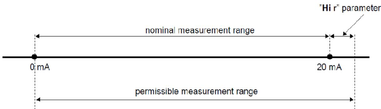
Fig. 6.2. definitions of measurement ranges in mode 0 ... 20 mA
