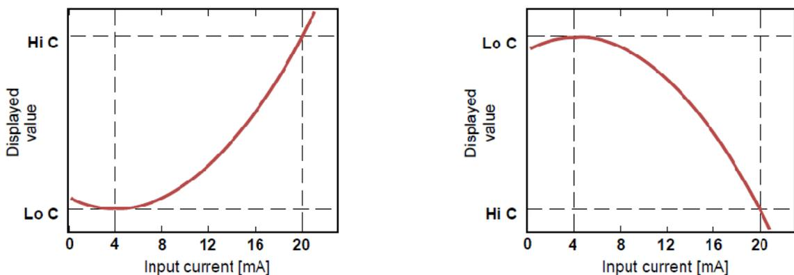
Fig. 9.2. normal („Lo C” < „Hi C”) and inverted („Lo C” > „Hi C”) characteristic
