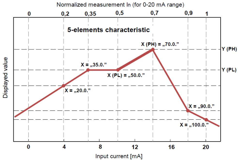
Fig. 9.17. Example of user defined characteristic
