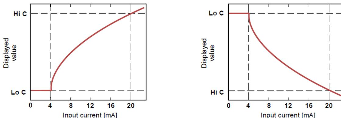
Fig. 9.3. normal („Lo C” < „Hi C”) and inverted („Lo C” > „Hi C”) characteristic
