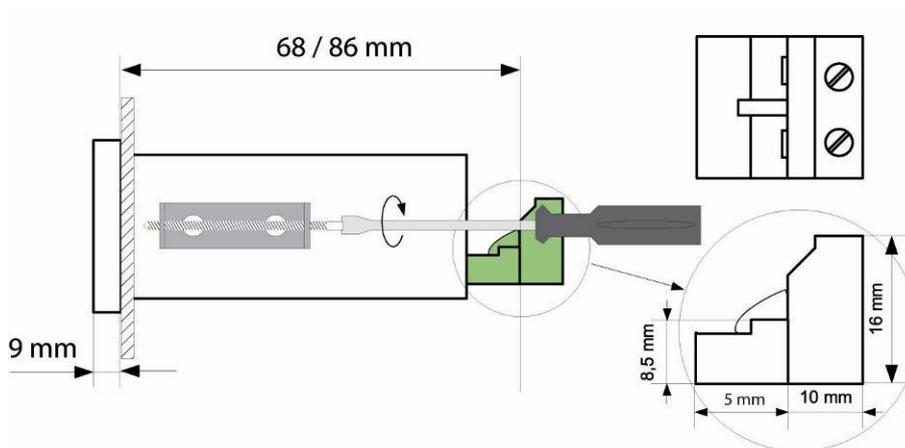
Fig. 4.2. installing of brackets, and dimensions of connectors
