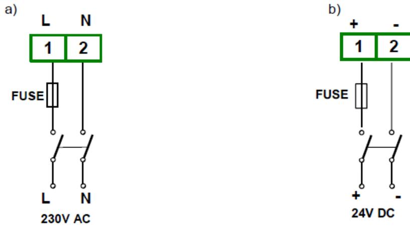
Fig. 4.6. connection of power supply
