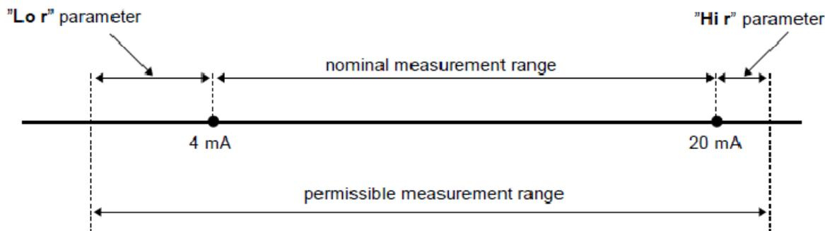
Fig. 6.1. definitions of measurement ranges in mode 4 ... 20 mA
