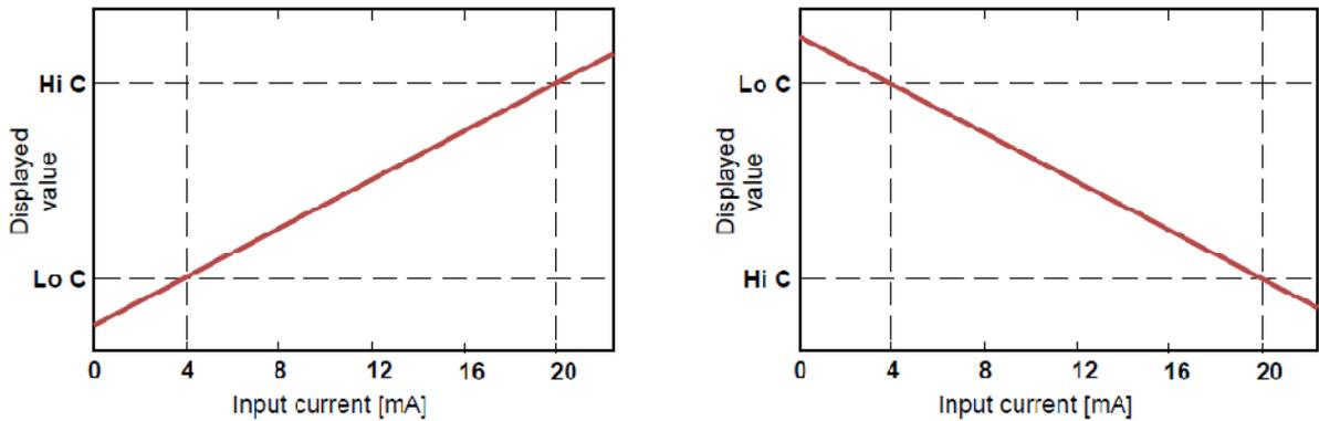
Fig. 9.1. normal („Lo C” < „Hi C”) and inverted („Lo C” > „Hi C”) characteristic
